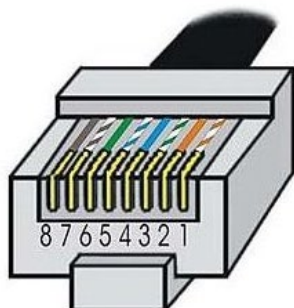
Fig 5.1 Pin Configuration for standard RJ45 plug
